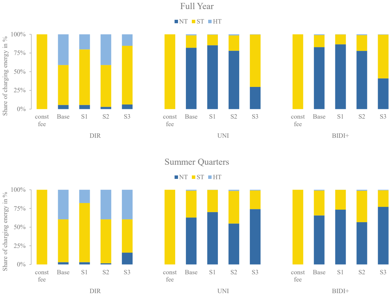
Figure 3: Average share of charging of the different levels of grid fee (NT, ST, HT) for constant grid fee (const fee) and different variable grid fee tariffs (Base, S1, S2, S3) for a household with one EV for different charging strategies (direct charging (DIR), smart unidirectional charging (UNI), and smart bidirectional charging (BIDI)), (a) full year, (b) 2 summer quarters
