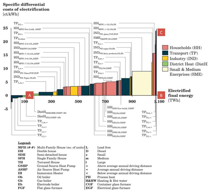
**Figure 2 – Merit-order of electrification 2050**
