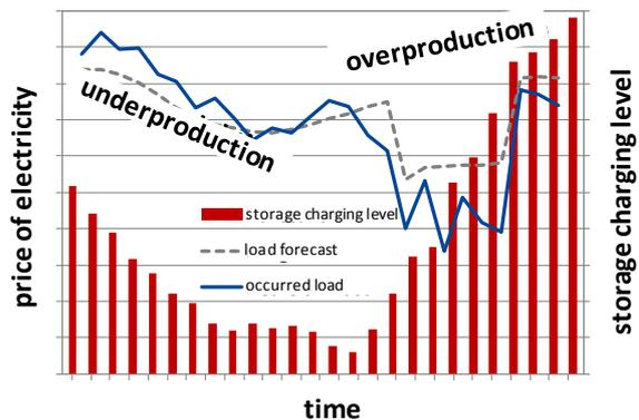
Figure 7: The balancing volume
