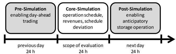
Figure 3 The sections of the simulation cycle
