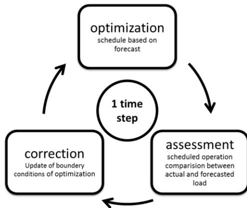
Figure 1: The closed loop of the simulation
