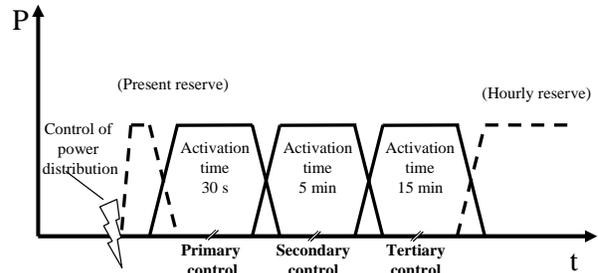
**Figure 2:** Load-frequency control phases and corresponding products.
