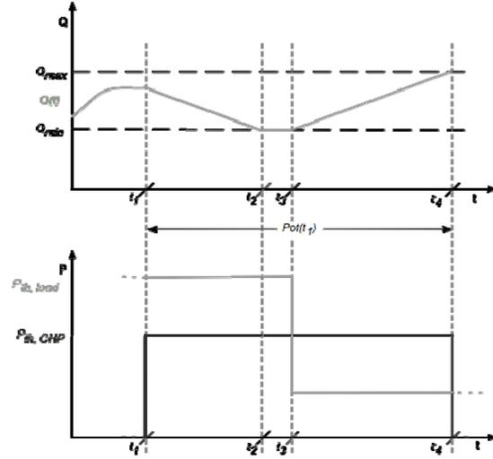
**Figure 4:** Variation in buffer storage with time, as simulated by the model
