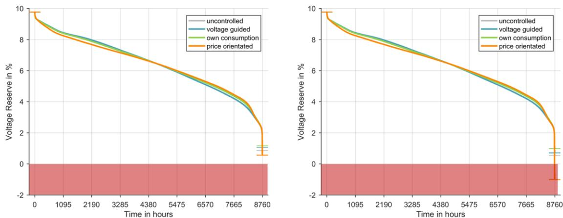
**Figure 8:** Duration curve of the voltage reserve of the different charging control strategies; left side: maximum charging power 11 kW, right side: 22 kW
