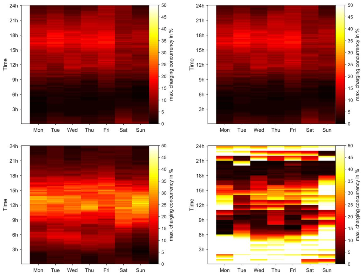
**Figure 6:** *Concurrency of charging events in dependency of the charging strategy (top left to bottom right: uncontrolled charging; voltage guided control; own consumption optimized control; price oriented control).*
