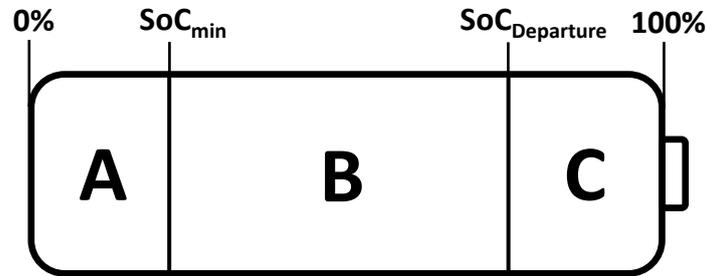
**Figure 2:** The battery of an electric vehicle can be divided into three fundamental sections in respect of its State-of-Charge
