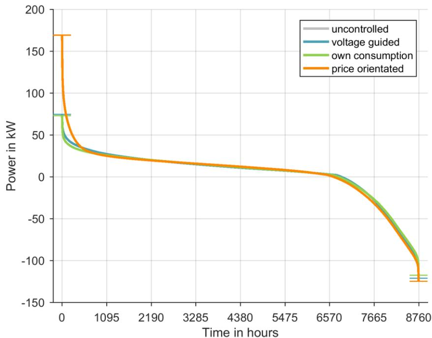
**Figure 7:** Power duration curve of the transformer for the different charging control strategies
