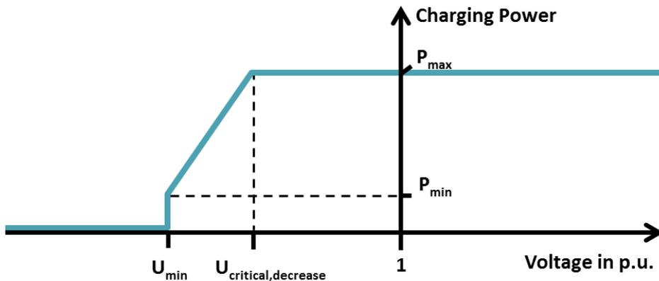
**Figure 3:** Permissible charging power for voltage guided control
