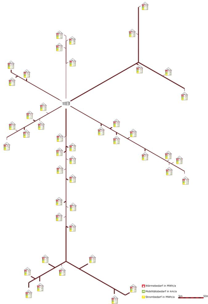
**Figure 5:** Type grid 4 represents a typical rural grid with 45 buildings which consist of one household each.
